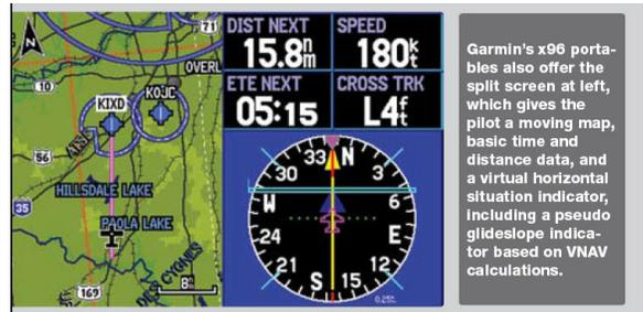
Garmin's x96 portables also offer the split screen at left, which gives the pilot a moving map, basic time and distance data, and a virtual horizontal situation indicator, including a pseudo glideslope indicator based on VNAV calculations.
